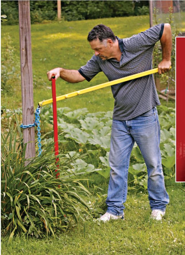
**Matt Baldwin, West Union, West Virginia, developed the BullPull post and shrub puller not only to make fence installation and repairs a simple process but also to remove shrubs.**
