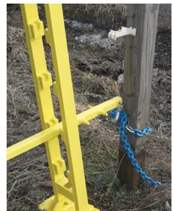
As the post comes out of the ground, you move handle up higher supports.
