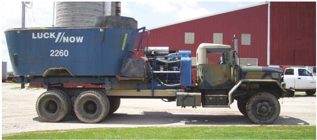
Dairyman Jay Boldt built this self-propelled feed mixer by combining parts from a military semi tractor and a Lucknow pull-type feed mixer.
