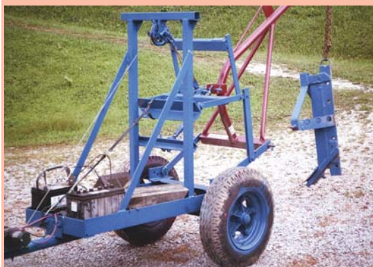
Electric winch is powered by a 12-volt car battery. Backup battery next to it is for emergency use. Boom pole is used to transport miscellaneous objects.
