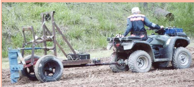
Home-built 3-pt. tool carrier rides on a pair of 15-in. wheels. An electric winch is used to raise and lower the 3-pt.
